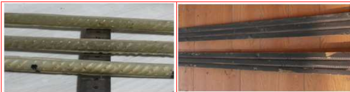
Fig. 1: Ripped 12mm bars with Crescent shaped lugs and double sets of plastic mold
